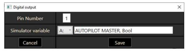
The bridge will continuously sync the output pin with the result of the simulator variable query. You can use either A: or L: variables that return a value of 0 or "not 0" or supply an RPN script that yields a 0/1 result (selection "S:"). For example, the configuration above could also be set up as
